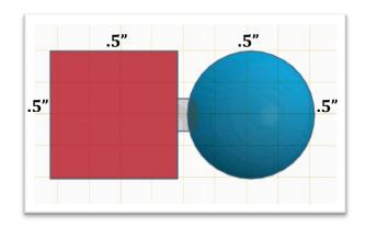
**Purpose**: Students will develop their CAD skills by successfully attaching a Cube to a Sphere with a peg. The peg sits in a hole that was formed in both shapes. This skill is the basis for the car that the students will soon create.
