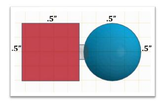
**Purpose**: Students will get to use and develop their CAD skills by successfully attaching a Cube to a Sphere with a Peg. The peg sits in a hole that was formed in both shapes. This skill is the basis for the car that the students will soon create.
